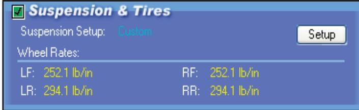
Despite its “simple” appearance, the *Suspension & Tires* component category is the most complex and comprehensive in FastLapSim. Click the *Setup* button to modify individual component specs.
