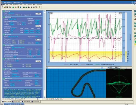
Race results are displayed in top-and-bottom screen windows (called panes). The main graph is a *Speed Combo Plot* along with *Lateral Acceleration*. Note the *DataZones™* within the main graph displaying vehicle speed bands (a *ProTools™* feature).
