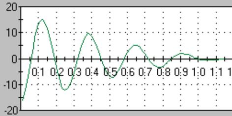
An under-damped suspension allows the spring to oscillate (compress and relax) more than necessary; letting the tire leave the road surface multiple times after encountering a bump. Under-dampening is often the result of the damper contributing insufficient force in bump, allowing the spring to store excessive energy which is returned to the wheel on rebound.
