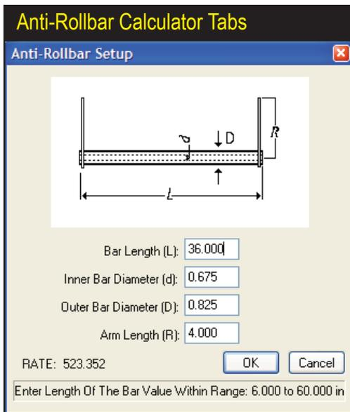
for a front or rear bar. The deflection force is generated by the difference in travel between the two sides of the vehicle. The compressed side will transmit a force through the bar that reduces the load on the opposite tire, producing a counter-roll force on the body at the bar attachment point. This causes the body to roll in the opposite direction (anti-roll).
