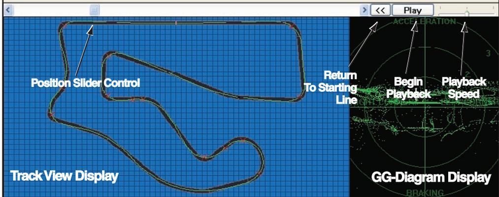
The Track View Display provides an overhead view of the track and the test vehicle. The position of the vehicle on the track is synchronized with the reticule on the main data display. Move through the course by dragging the graph reticule, moving the Position Slider, or by pressing the *Play* button just above the *GG-Diagram Display*.
