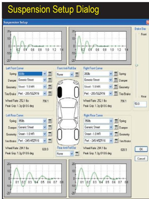
**Suspension Setup:** This menu presents several "prepackaged" choices of entire suspension setups, including selections for suspension design, spring rates, sway bars, shocks, tires, and brakes. Using these upper-level choices you can quickly evaluate "stable" system packages on a variety of vehicles and tracks. And if you wish to modify component groups to test their effect on vehicle handling and performance, simply click on the **Setup** button to open the Suspension Setup dialog box.
