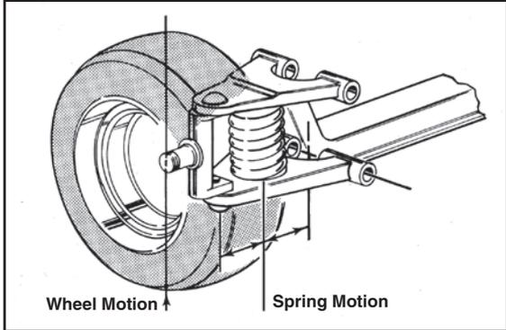
fields in the **Spring Geometry** group, the **Motion Ratio** for the suspension will be calculated. Similarly, when the fields in the **Damper Geometry** group have been completed, the **Motion Ratio** of the damper will be calculated.
