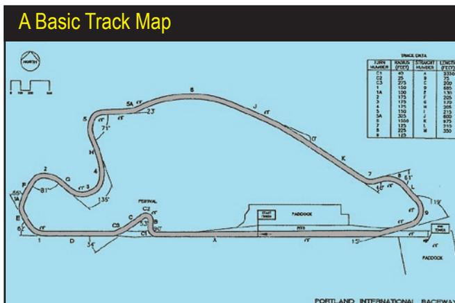
The first step in building a real-world racetrack in the Track Editor is to base your “construction work” on a detailed drawing of the Raceway. This drawing was compiled from published sketches and track data (scale is 300-foot = 1-inch). Always try to obtain an overhead track map, aerial photo, or any other descriptive data of the track before you attempt modeling in the Track Editor.
