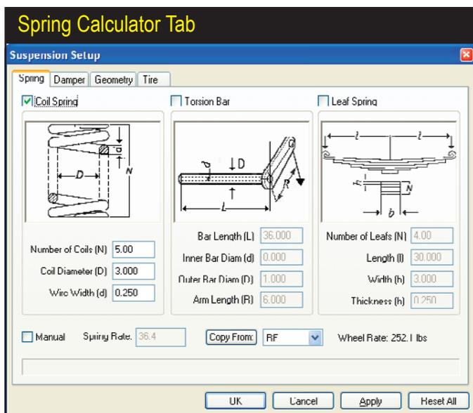
*The Spring Calculator Tab* lets you select three types of spring systems for each wheel: Coil Springs, Torsion Bars, or Leaf Springs. When you select one of the three spring types, the related fields for that spring are activated. Enter the required specifications, and the spring rate will be calculated and displayed in the **Spring Rate** field. (Alternatively, you can directly enter a spring rate by clicking the **Manual** box.)
