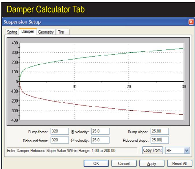
*The Damper Calculator Tab displays the results of “shock-dyno” test curves. The curves indicate how the damper resists movement in both bump and rebound. Modify the bump and rebound curves by entering custom specifications in the Force, Velocity, and Slope fields.*
