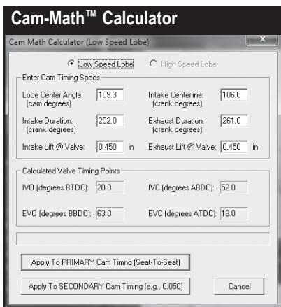
The **CamMath™ Calculator** is just one of the tools you can use to help model engines in Dymotion6. Enter readily available cam duration and centerline values and the Calculator will determine valve-event timing needed to complete the simulation.
