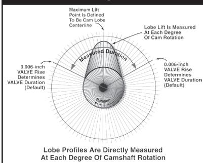
**Lobe Profiles Are Directly Measured At Each Degree Of Camshaft Rotation**
