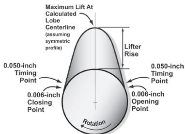
**10-Point Cam Timing Is Derived From Seat-To-Seat and 0.050-Inch Opening and Closing Points, Plus The Maximum Lift Of Each Lobe**
