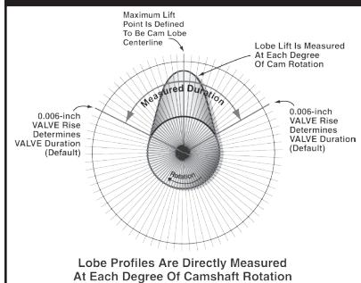
Profile data is made up of lobe-lift data recorded at, usually, each degree of camshaft rotation (by installing the cam in a special measuring fixture). Dynomation6 can use this data to very accurately determine valve positions at any point during the simulation.
