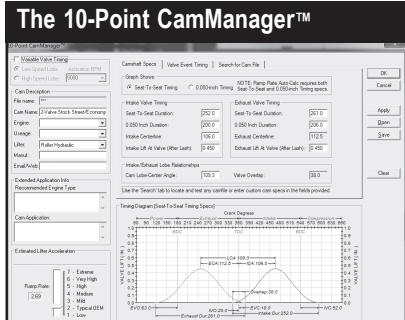
**The 10-Point CamManager** is the “central clearing house” through which you can load, save, and search for 10-Point CamFiles.
