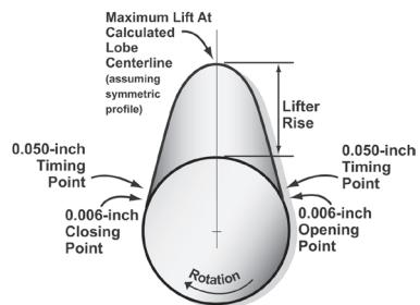
**10-Point Cam Timing Is Derived From Seat-To-Seat and 0.050-inch Opening and Closing Points, Plus The Maximum Lift Of Each Lobe**
